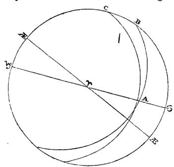
In the oblique spherical triangle ABC are given the angle ACB, the co-longitude. AC the co-latitude, and AB the co-declination of the planet or star, to find its right ascension, viz. the co-angle at B.
