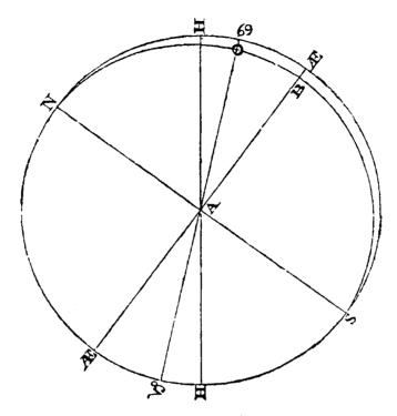
In the right angled spherical triangle A B  $\odot$ , A  $\odot = \odot$ 's longitude from the nearest equinoctial point, and the angle B A  $\odot = 23^{\circ}$  28' nearly,—the obliquity of the ecliptic, are given to find B  $\odot$  = his present declination.
