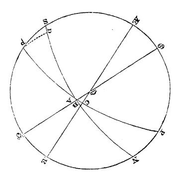
In this diagram A represents a star in a southern sign, with southern latitude also.  $\triangle$  B is its longitude, B A its lat. Then in the oblique angled spherical triangle A S p we have A S = the complement of its lat. p S, = the obliquity of the ecliptic, with the angle p, S D = its longitudinal distance from the solstitial point  $\mathcal{V}$ . To find C A the star's declination. For which we have the following rules:—
