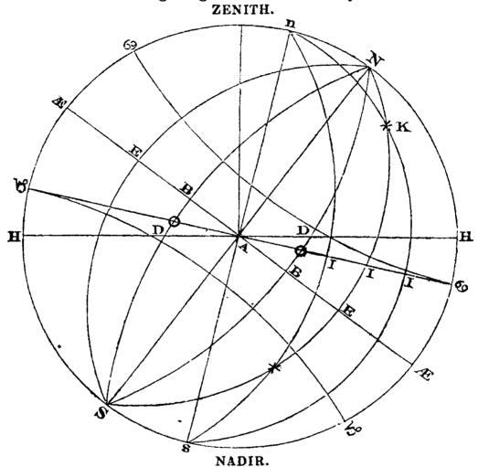
Construction.—With the chord of 60 degrees describe the circle Zenith H, Nadir H, and draw the diameter H H. Take the chord of 53 26, and set it from H to N; then through the centre of the circle draw N A S.
