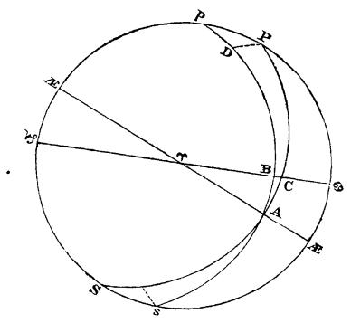
In the above diagram let A represent the position of a star in a northern sign with south latitude;  $\gamma$  B is its long. from  $\gamma$ . B A its latitude south, and C A it declination north. Then in the oblique angled spherical triangle A s S, are given A s = the complement of the star's lat.
